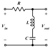
a. Determine an expression for the voltage transfer function,  $\mathbf{V}_{out}/\mathbf{V}_{in}$ . Also, determine expressions for the magnitude and the phase angle of that transfer function.
